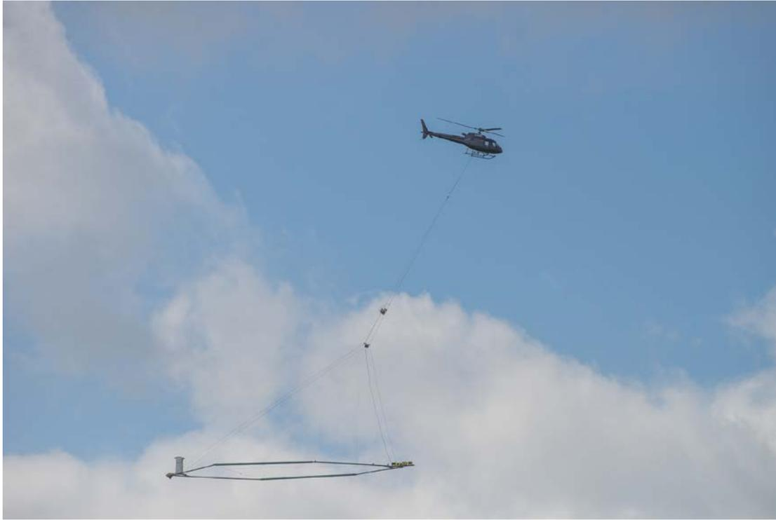
**Figure 3** - SkyTEM Electromagnetic System (courtesy of SkyTEM ApS)
