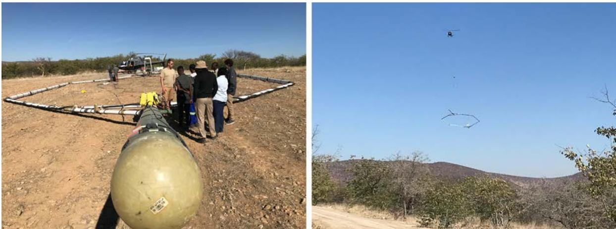
**Figure 1** – Namibia Critical Metals geological team being briefed on the SkyTEM system’s operation (left). Magnetometer in foreground; EM coil is 28 m in length and 16.5 m wide. System is flown with an AS350 helicopter operated by Savannah Helicopters shown flying at Kunene on right.
