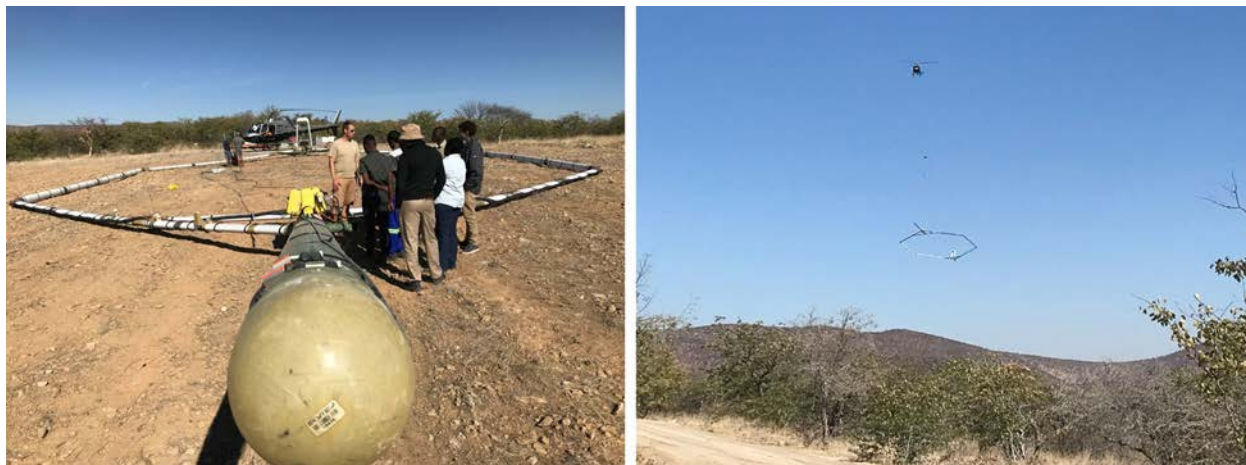
Figure 5 – Namibia Critical Metals geological team being briefed on the SkyTEM system's operation (left). Magnetometer in foreground; EM coil is 28 m in length and 16.5 m wide. System is flown with an AStar 350 helicopter operated by Savannah Helicopters shown flying at Kunene on right.
