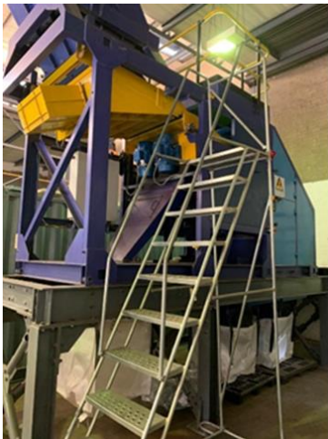
Figure 4. Rados test facility in Pretoria with observation deck to XRF feed hopper on left and final calibration algorithm showing correlation between Rados analysis for yttrium and %TREO
