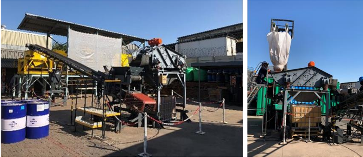
Figure 5. IMS test facility in Johannesburg showing feeder conveyor to XRT sorter on left and Lofdal bulk sample ready for screening on right
