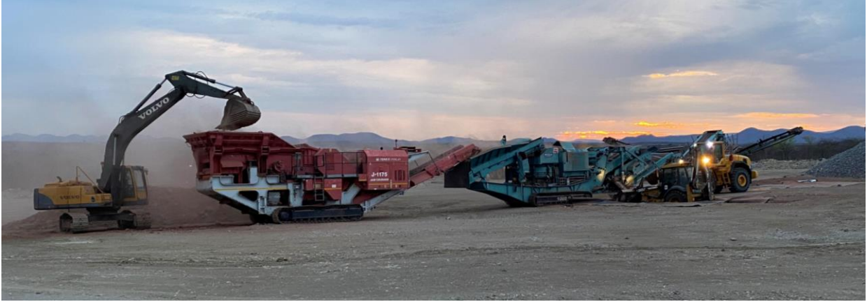
Figure 2: Crushing and screening of the bulk samples by Gecko Mining
