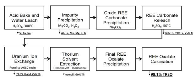
Figure 1: Hydrometallurgical process flowsheet developed in 2021 using Lofdal flotation concentrate
