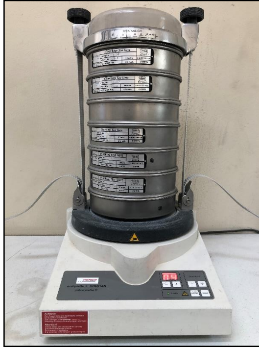
Figure 2: Fritsch Analysette 3 Spartan at Geolabs Global
