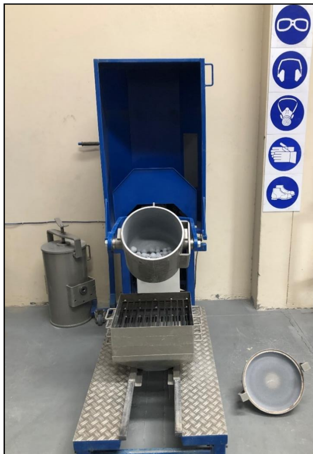
Figure 1: Bond Ball Work Index tester at Geolabs Global
