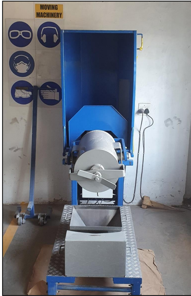
Figure 3: Bond Rod Work Index tester at Geolabs Global
