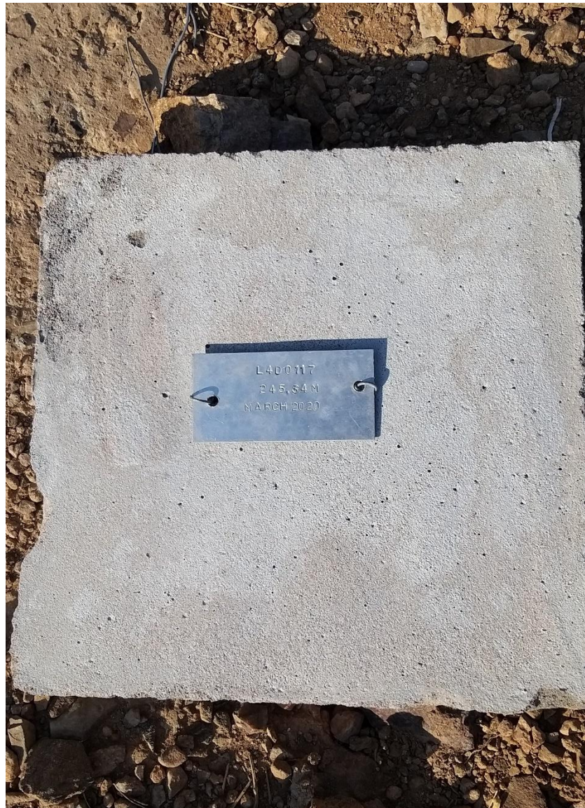
Figure 10-5 Concrete Plinth over Capped Drillhole L4D017
