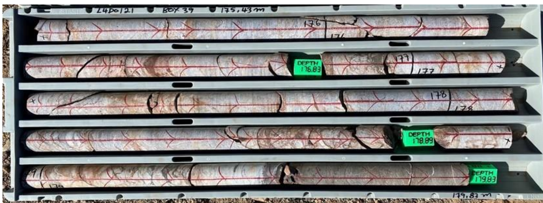
Figure 10-4 Drillers' Metre Marks, measured Metre Marks and Orientation Lines on Uncut Core
