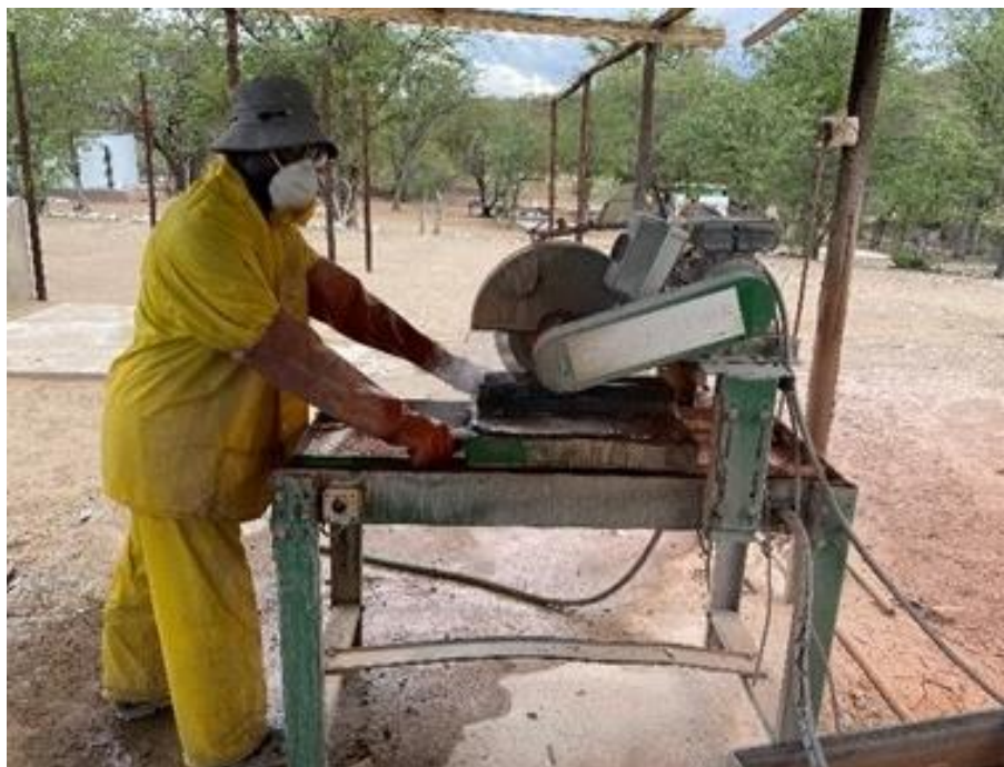
Figure 11-3 Core Cutting Device
