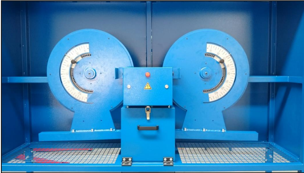
Figure 6: Bond Low Energy Impact Test at Geolabs Global
