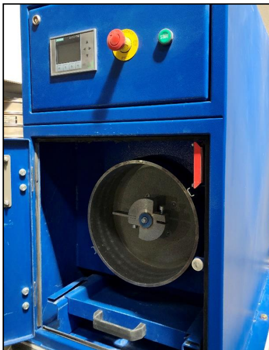
Figure 4: Bond Abrasion Index tester at Geolabs Global
