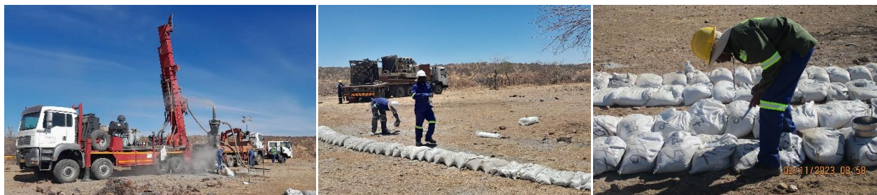
Figure 1: Impressions from the final infill drilling campaign at Lofdal: Drill rig of Prinsloo Drilling allowing for precise high-quality RC drilling to over 400 m depth at central Area 4 deposit (left), sample line up and recording (centre), and gamma logging of the first 360 m hole by Gecko Exploration on Thursday, 2 November 2023.
