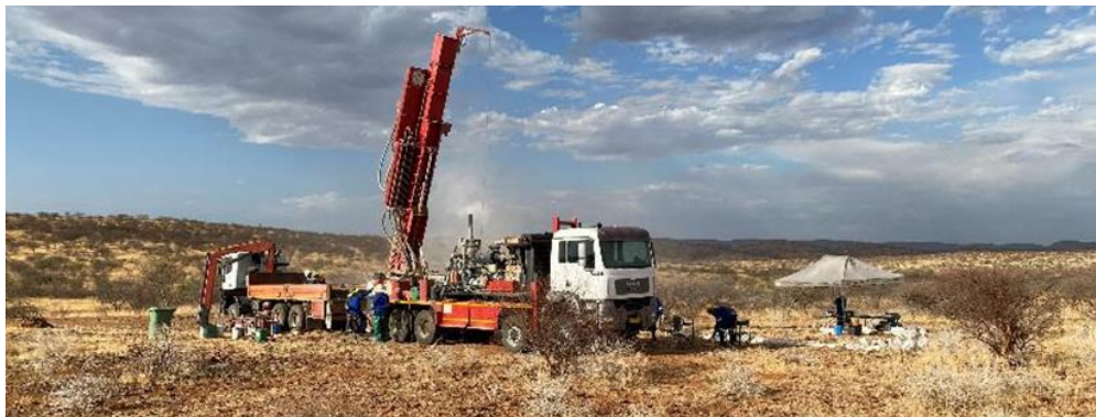
Figure 1: RC drill rig of Prinsloo Drilling at the final drill position in the western part of Area 4
